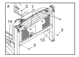
With the help of a second person, carefully raise the Uprights (13, 14) to the position shown. Carefully pivot the Hood (41) off.
